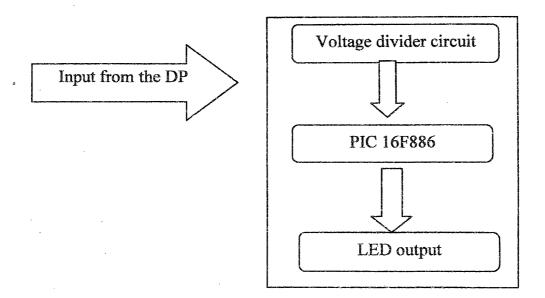
Figure 1: The block diagram of the free loops identify unit.
