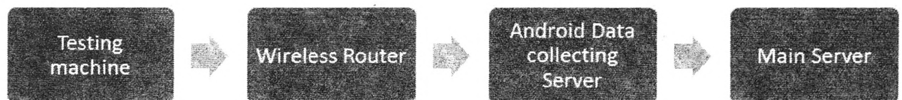
Figure 1: The block diagram of the harness testing and live updating system
