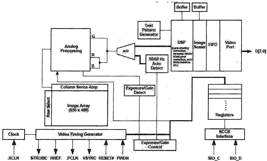
Figure 1: Functional Block Diagram of OV7670
