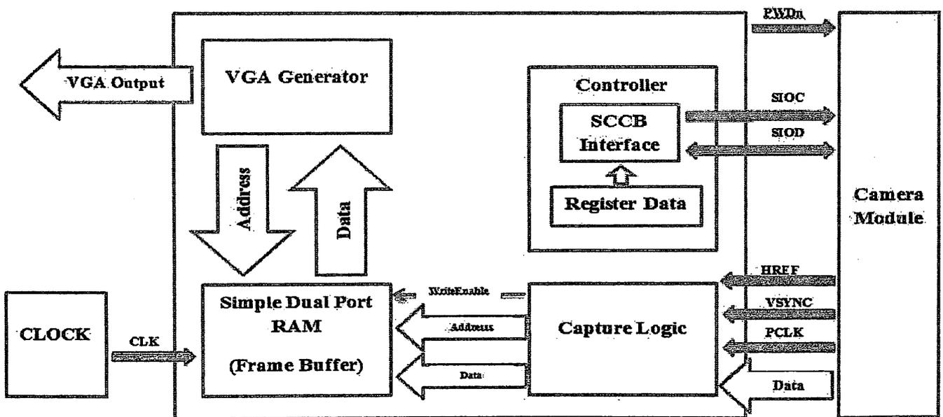
Figure 2: Block diagram of interfacing camera module with FPGA
