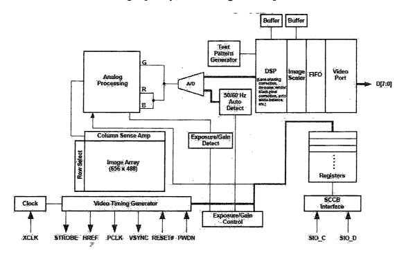
Figure 1: Functional Block Diagram of OV7670
